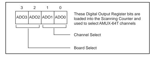
Figure 5-2. Scanning Counter Control Bits
