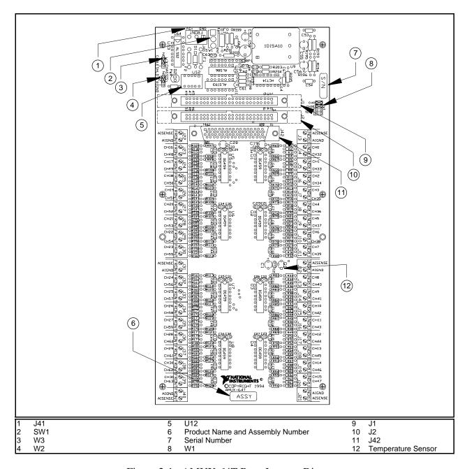
Figure 2-1. AMUX-64T Parts Locator Diagram
