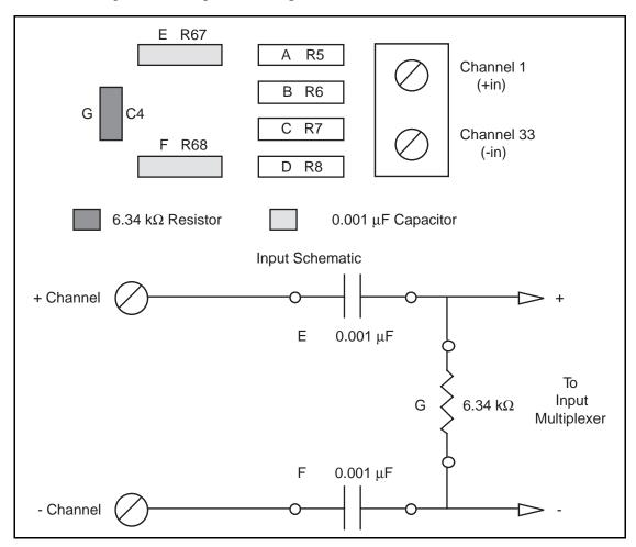
Figure 4-6. Highpass Filter on Differential Channel 1
