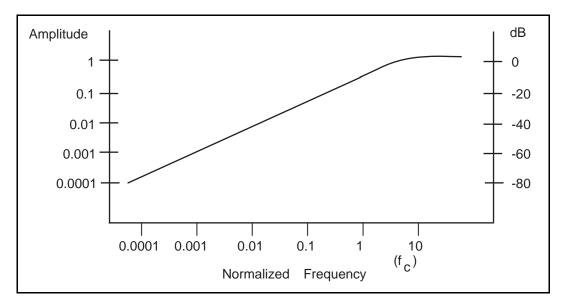
Figure 4-5. Normalized Frequency Response of Highpass Filter
