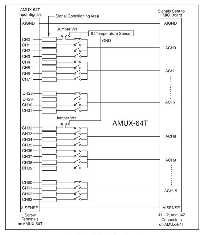
Figure 3-1. AMUX-64T Signal Routing
