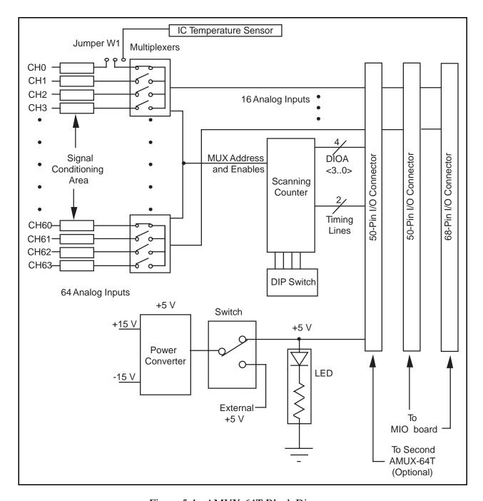
Figure 5-1. AMUX-64T Block Diagram
