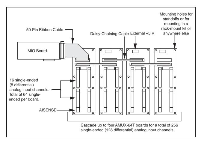
Figure 2-2. Daisy-Chaining Multiple AMUX-64T Boards
