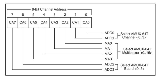
Figure 5-3. AMUX-64T Channel Address Mapping
