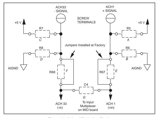
Figure 4-1. Onboard Equivalent Circuit
