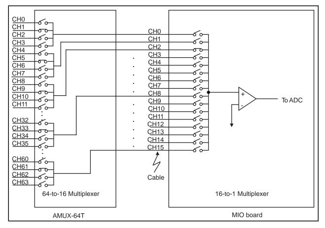
Figure 5-4. Two-Level Multiplexer Arrangement Showing Channel 9 Selected
