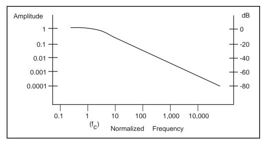
Figure 4-3. Normalized Frequency Response of Lowpass Filter
