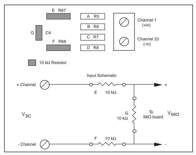
Figure 4-7. Attenuator for Use with Differential Inputs
