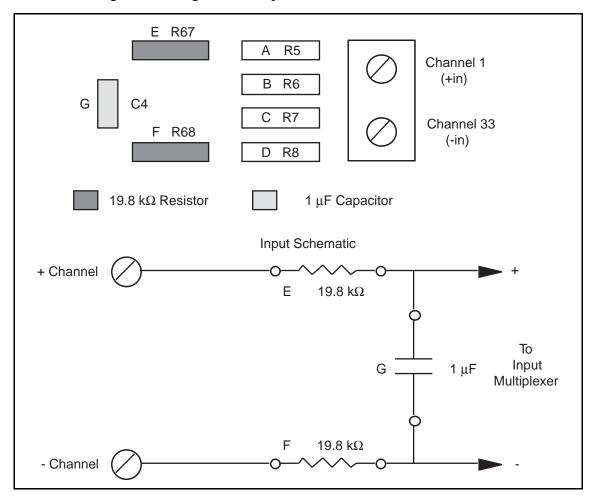
Figure 4-4. Lowpass Filter on Differential Channel 1
