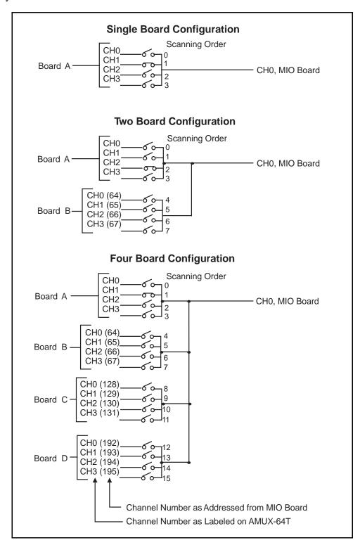
Figure 5-5. Scanning Order for Different AMUX-64T Board Configurations
